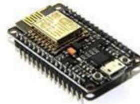
Fig. NodeMCU Development Board
